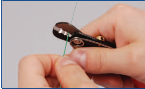
1.4 Strip Off Cladding
