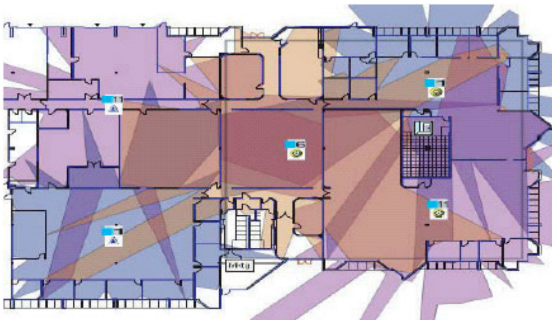
Figure 6: Picture: support for third-party APs includes the ability to model the RF signal contours of those APs. This view shows two third-party APs modeled on the left and three mobility points on the right. [12]
