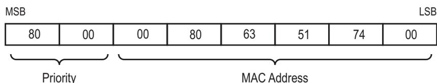
Figure 6: Bridge identifier, example (values in hexadecimal notation)
