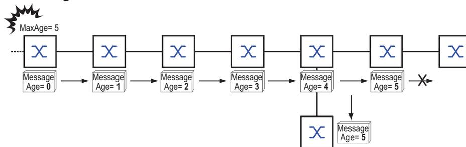
Figure 10: Transmission of an STP-BPDU depending on MaxAge
