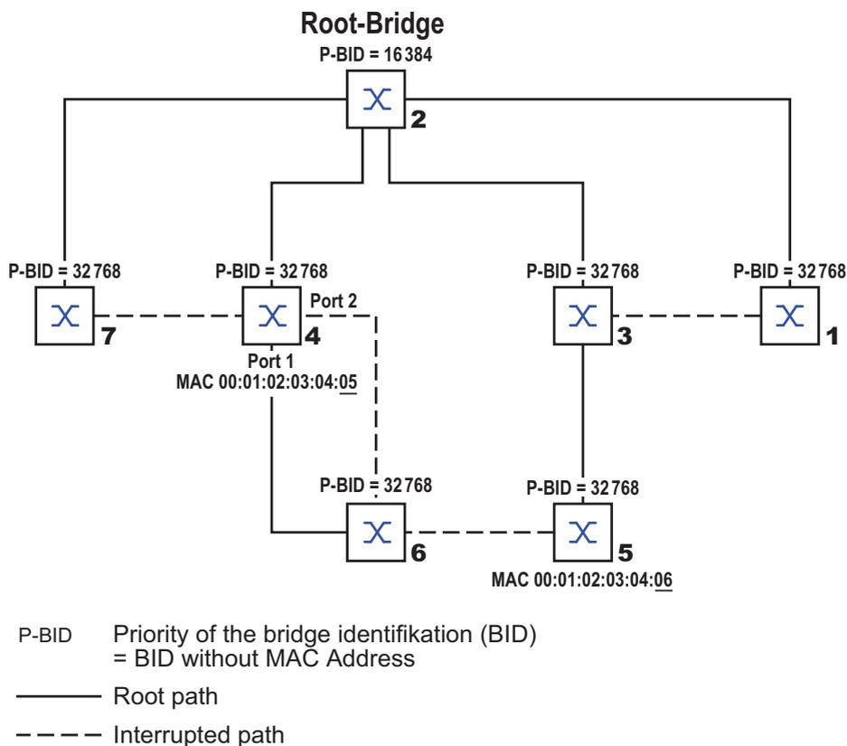
Figure 14: Example of manipulating the tree structure
