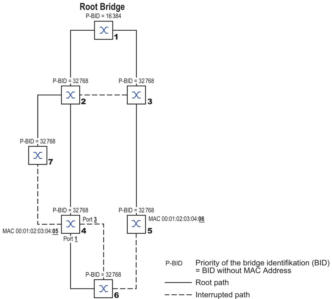
Figure 12: Example of determining the root path
