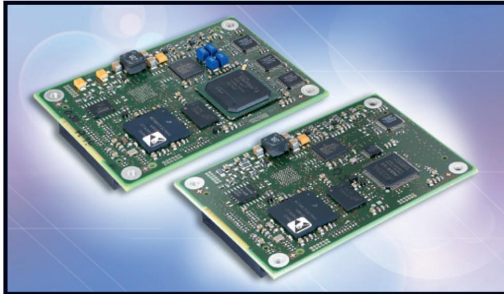
**The New Embedded Ethernet EES20 and EES25 Switches from Hirschmann™ Combine the Functional Scope of a Powerful Managed Switch With Interruption-free Redundancy Protocols and Precise Synchronization.**
