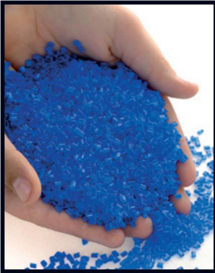
The use of non halogenated materials in both the cable insulation and the cable jacket is essential.
