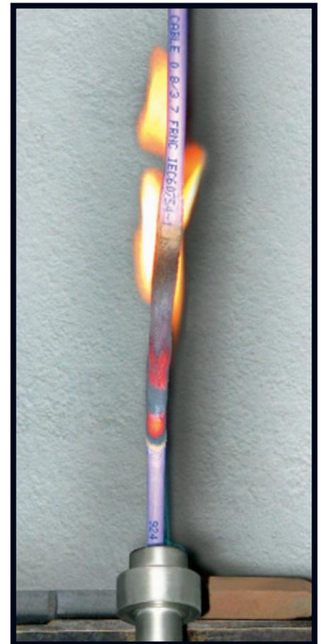
IEC standard 60332-1-2 Single Wire Flame Test
