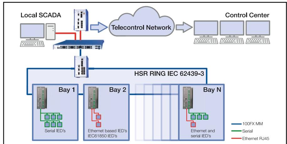
With HSR technology substations networks can be expanded just chaining bays without affecting the current network.
