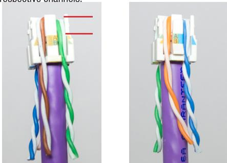
Pairs should lay flat (side by side) between the red lines. Verify your white conductors are all on the outside.
