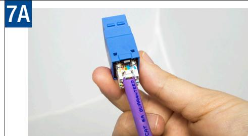
Align the rear jack latch with the latch on the cable manager and snap on your RJ45 housing. The terminated jack is now ready for testing.
