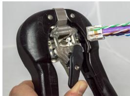
Insert the terminated core (cable manager and cap) into the tool until the middle latch returns to the center.
