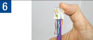
Align the contacts of the cap with the wired cable manager and push until it snaps down.
