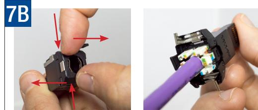
Open the rear doors of the RJ45 plug by squeezing vertically on the pins and pulling your fingers apart.
