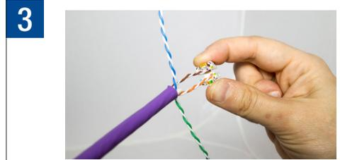
Locate the brown box on the bottom of the cable manager. Insert the brown pair and green (for T568A) or orange (for T568B) pair through the holes and begin sliding the manager down the cable
