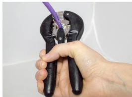
While holding the cable with one hand, compress the handles to complete your termination
