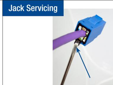
To remove, press down on the latch with a small screwdriver (or Belden release tool) and pull the cable out
