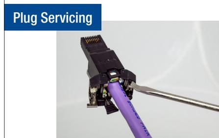
To remove, open the rear doors by squeezing the upper and lower pins. Lift on the latch with a small screwdriver (or Belden release tool) and pull the cable out
