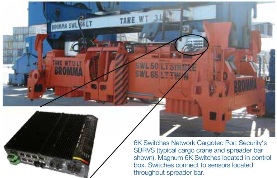
6K Switches Network Cargotec Port Security's SBRVS (typical cargo crane and spreader bar shown). Magnum 6K Switches located in control box. Switches connect to sensors located throughout spreader bar.
