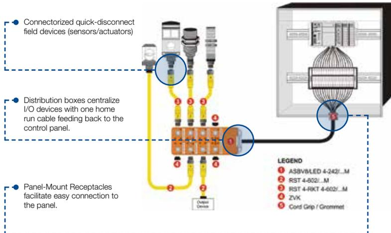
**Figure 1:** Enclosure-less I/O strategies provide multiple benefits including less cable to run initially and easier troubleshooting and faster fault resolution when alarms occur.
